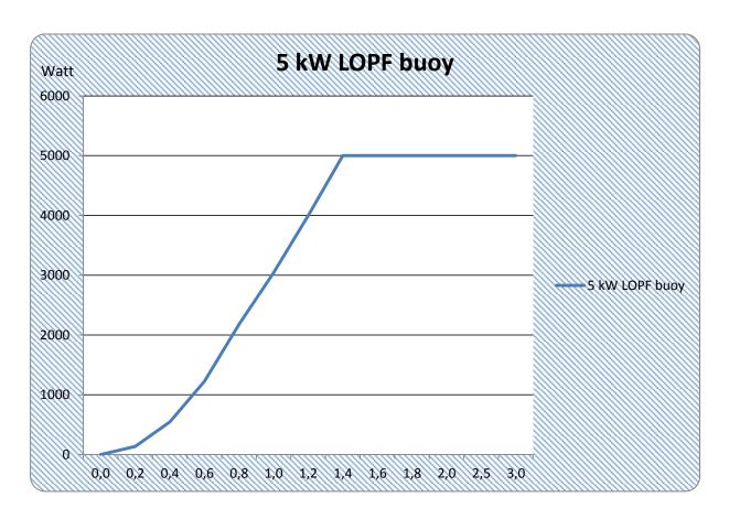
The graph represents the power output in Watt's versus Hs (m), significant wave height.
